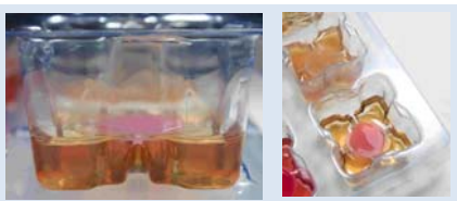
Figure 1. 24-hour S. aureus biofilm supported on a 25 mm Anodisc in contact with growth medium in a deep 6-well culture plate (biofilm is stained pink for clarity in these photographs)
