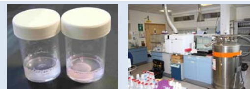
Figure 4. Dissolution of residual biofilm and the ICP-MS used to analyse samples
