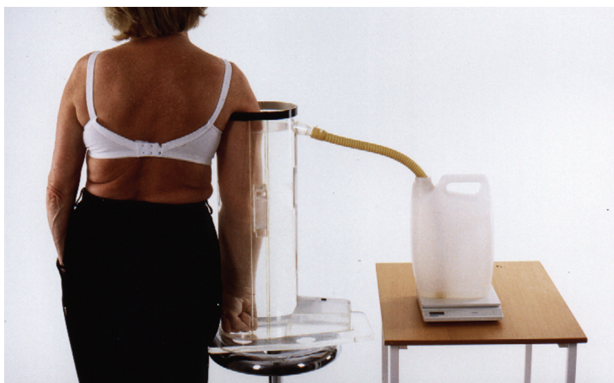
Figure 2. Arm volume measurement with water displacement method.
