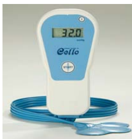
Fig 2: Interface pressure sensor 'Cello', co-developed with a medical company. The soft sensor pad can safely measure the pressure produced between body and support surface
