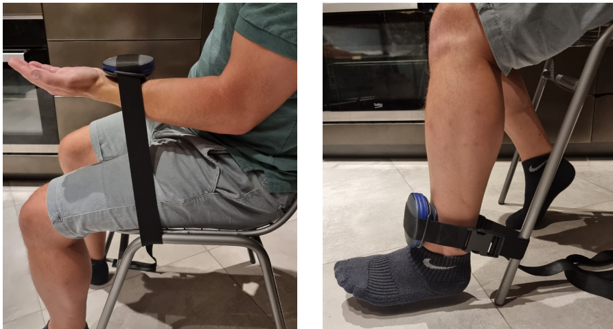
Figure 1. Left: The upper limb strength measurement technique fixed at the chair. Right: The lower limb strength measurement technique fixed at the leg of the chair.
