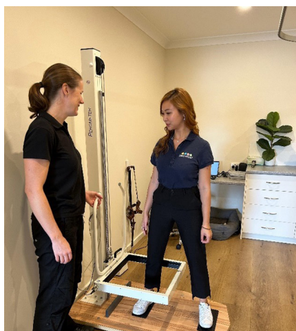
Figure 6 – A photo of the stand-up perometer. Kate is standing in front of the perometer looking at a woman standing full clothed inside the perometer. The woman is demonstrating how her right leg would be measured.
