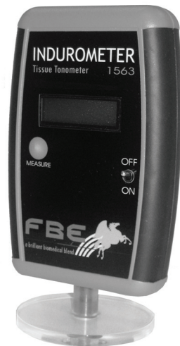
Figure 2. Indurometer, manufactured by FBE Pty Ftd, Australia. The transparent reference plate of the device rests on tissue.
