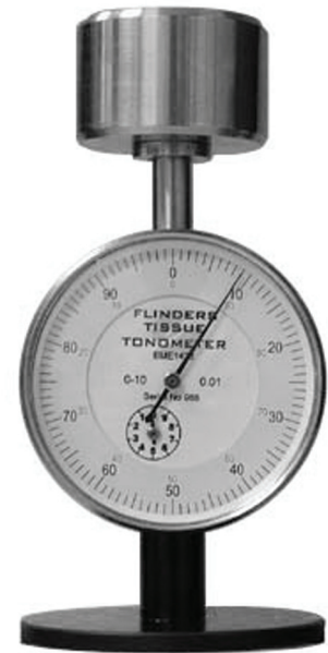
Figure 1. Mechanical tonometer, manufactured by Biomedical Engineering, Flinders Medical Centre, Australia. The black reference plate of the device rests on tissue.
