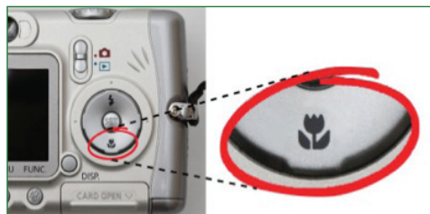
Figure 1. Macro function – identified by the flower icon highlighted here – switches the camera into a close-focus mode, allowing more detailed images of the wound to be taken.
